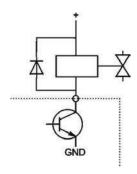
Fig. 4-30: Suppressor diode for inductive loads.
